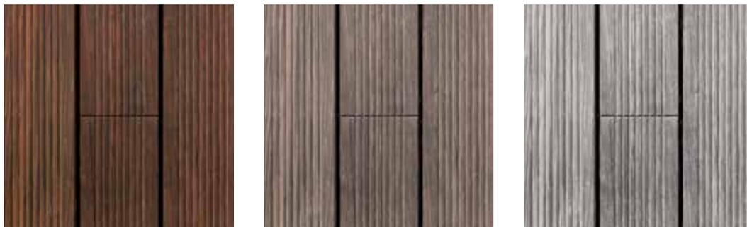
Gradual graying of MOSO® Bamboo X-treme® over time: new, non-weathered decking (left), after 3 months of weathering (middle) and after 18 months of weathering (right).
