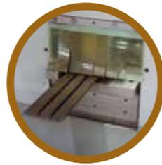
split the Moso bamboo stems, remove the skins and crush the strips into strands
