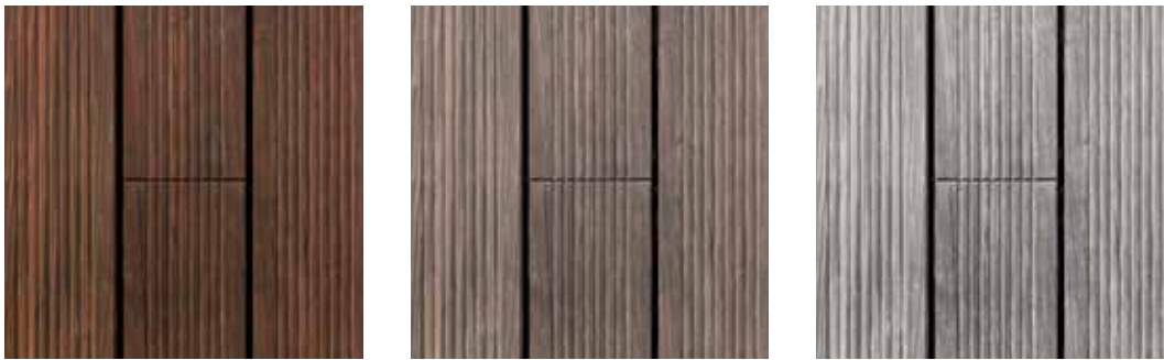
Gradual graying of MOSO® Bamboo X-treme® over time: new, non-weathered decking (left), after 3 months of weathering (middle) and after 18 months of weathering (right).
